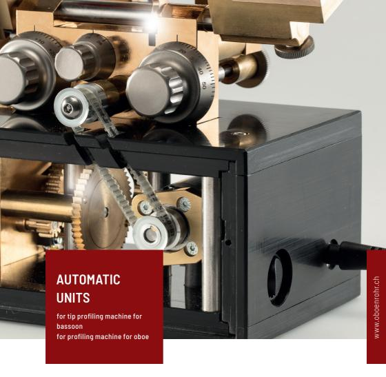
Automatically coordinated regular movements of the axis and the sledge allow for highest exactness of the scrape. Amazing precision - high-grade materials and durability.
