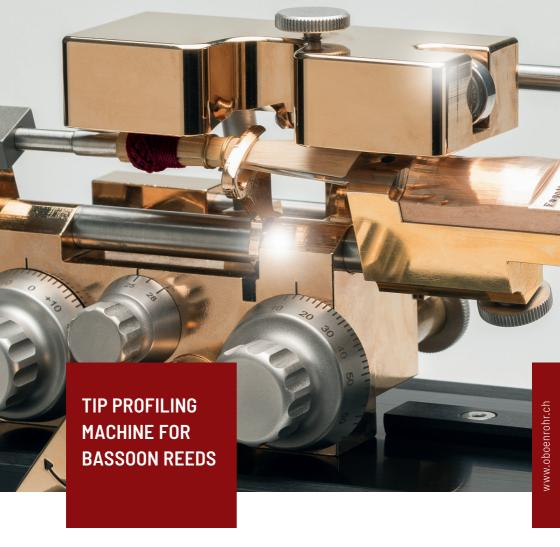
Precise scraping of highest quality, consistent reproduction with little time necessary. Length of the scrape up to 28mm. Simple, user-friendly operation: A mature product of years of development.
